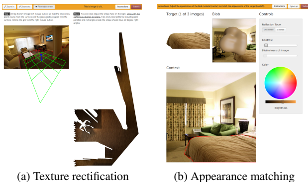
Figure 3: (a) Stage 7: Rectifying planar textures interface. This figure shows a successfully completed task, where the perspective grid on the left appears to lie flat against the surface, and the texture, shown on the right, is correctly rectified. (b) Stage 8: Interface for appearance matching to recover material parameters.
