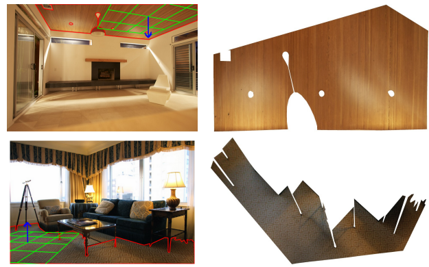
Figure 6: Example rectified textures. Left: original photographs with segmented surface highlighted and user-specified surface normal. Right: rectified texture with provided surface normal.
